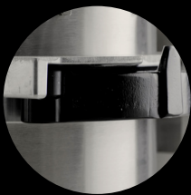
Automatic bowl lock and magnetic bowl detection
