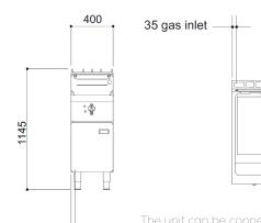
The unit can be connected at the rear or from below
