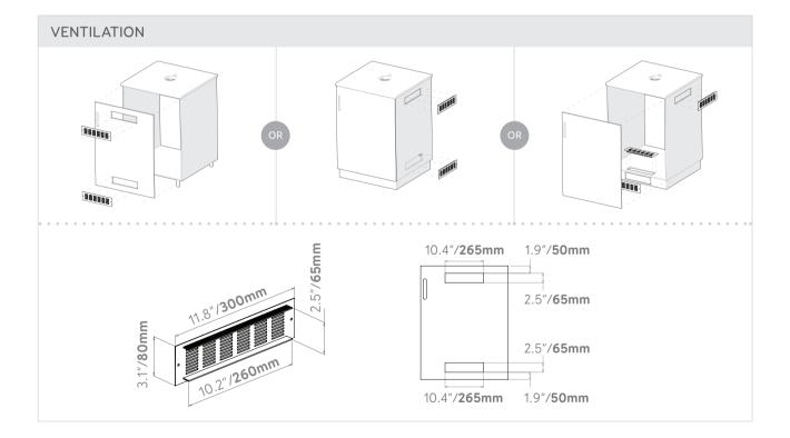
PLEASE NOTE It is essential to allow for two ventilation points when installing FRIIA. Vents are not supplied. Where possible, we recommend removing the back of your cabinet.
