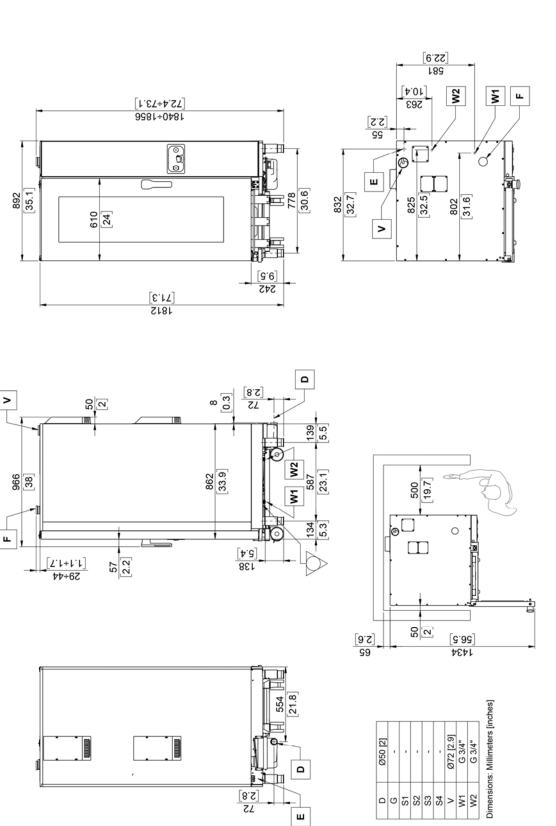
For model with steam generator Equipotential connection  $\overline{\mathbf{b}}$ Steam vent and cooking chamber pressure drop safety device Steam generator fumes exhaust Softened water inlet Water inlet S4\* > ž W2 Cooking chamber fumes exhaust Cooking chamber fumes exhaust Steam generator fumes exhaust Gas inlet Ċ S1 S2 S3\* Technical compartment cooling air intake Electric power supply cable inlet Cooking chamber air intake Liquid discharge ۵ ∢ ш ш
