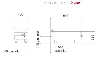
The unit can be connected at the rear or from below
